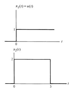
b) Express  $x_2(t)$  in terms of  $x_1(t)$  and then by taking advantage of the linearity and time-invariance properties, determine how  $y_2(t)$  can be expressed in terms of  $y_1(t)$ . Verify your expression by evaluating it with  $y_1(t)$  obtained in part (a) and comparing it with  $y_2(t)$  obtained in part (a).
